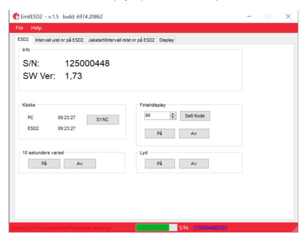
The green bar at the bottom of the screen indicates the battery voltage, while "S/N" means serial number. The serial number and firmware version are also displayed in uppercase letters at the top of the screen.
