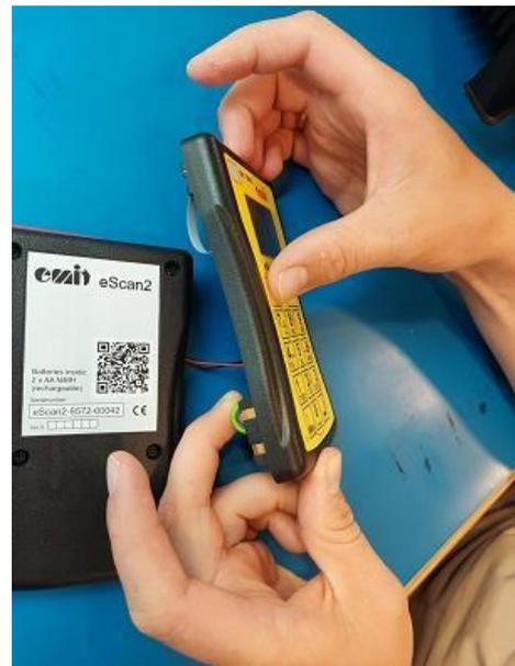
5. Press ON key and at the same time set the battery in place (USB must be disconnected!)
