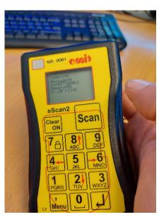
6. Fasten the four screws, put the rubber cover on and charge eScan2
