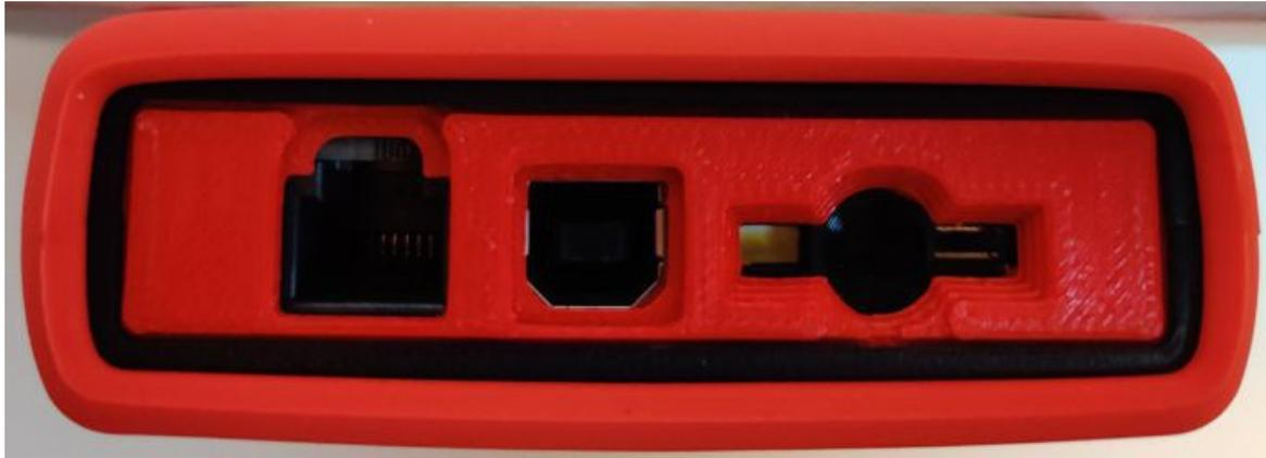
The port on the left is a serial port, which is used for connecting various external equipment, such as serial printer, starter gate, photocells, etc. The port in the middle is used to connecting an USB cable - to transfer data to PC with suitable results program, and for charging eScan2. The slot on the right is used for reading QR codes and barcodes.
