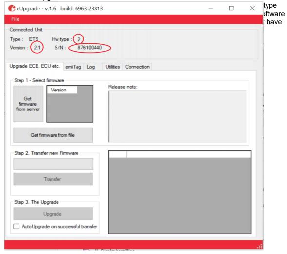
If eUpgrade doesn't show any information, check that the ETS2 is properly connected and that the USB-driver has been correctly installed in Windows.
