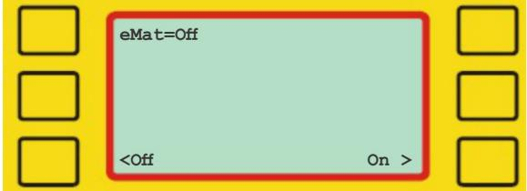
Press 'On' to enable eMat – which is used in biathlon to match start numbers/targets. Defaults setting is 'Off'.
