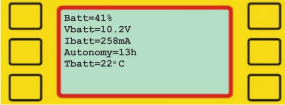
The power info menu shows how much battery capacity that is left on the first line. The second line shows how many volts the battery has, while the third line
