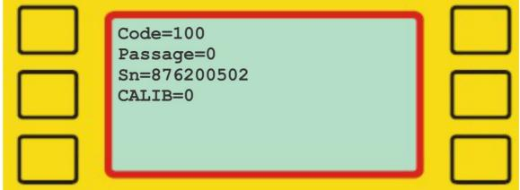
The general info menu shows which code the ETS2 is set to on the first line. The second line shows how many passings it has recorded in the current session. The serial number is shown on the third line, while calibration status is shown on the forth line.
