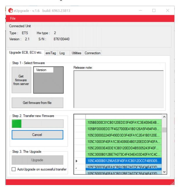
Wait until eUpgrade has finished transferring the new firmware version, and click the 'Upgrade'-button. After approximately ten seconds the ETS2 will restart with the new firmware version.
