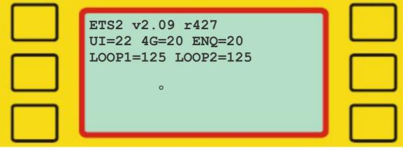
The versions info menu shows the version number for the ETS2 on the first line. The second and third line shows the version numbers for various sub-processes.
