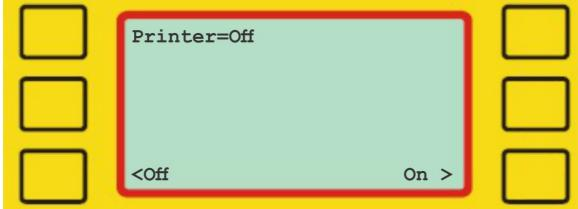
Press 'On' to enable printing, if the ETS2 has a printer installed. Default setting is 'Off\*.
