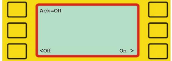
Normally 'Ack' (acknowledgement) should be turned on, which is the default setting. This means that the emiTags stop resending data after receiving 'Ack' from the ETS2. Set 'Ack' to off only when the ETS2 is used in combination with another ETS2.
