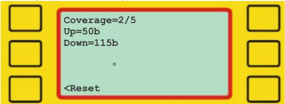
The modem info menu shows the coverage on the first line (0= no coverage, 5= excellent coverage), while the second and third line shows how much data has been uploaded and downloaded. Press 'Reset' to reset this information.
