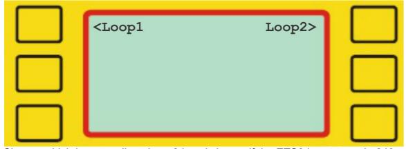
Choose which loop to adjust. Loop2 is only in use if the ETS2 is set to code 248.
