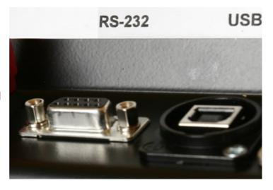
The first time you connect the ETS2 to a PC with an USB cable, you might have to install two drivers; 'USB Serial Converter' and 'USB Serial Port'. Normally this is done automatically, depending on the PC's operating system.
