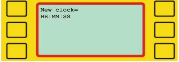
Use the numeric keys to set a valid time between 00:00:00 and 23:59:59. Start the clock by pressing 'Enter' or by short-cutting the 'START/SYNC'-input.
