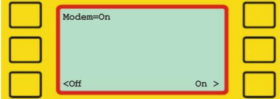
Press 'On' to enable the modem, if the ETS2 has a modem installed. Default setting is 'Off'.
