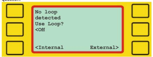
Answer "Off' if you don't want to use a loop with the ETS2. Choose 'Internal' if you want to use the internal eLine loop. Note that this loop is mounted at the bottom of ETS2, and the range is merely three meters. Answer 'External' if you have connected an external eLine loop to the 'LOOP 1' port on the ETS2.
