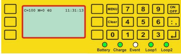
The display of the ETS2 has seven available lines and up to 20 symbols. Three keys on each side of the display control the various menu choices. In addition the keypad has numerical keys and comma, plus four set keys.
